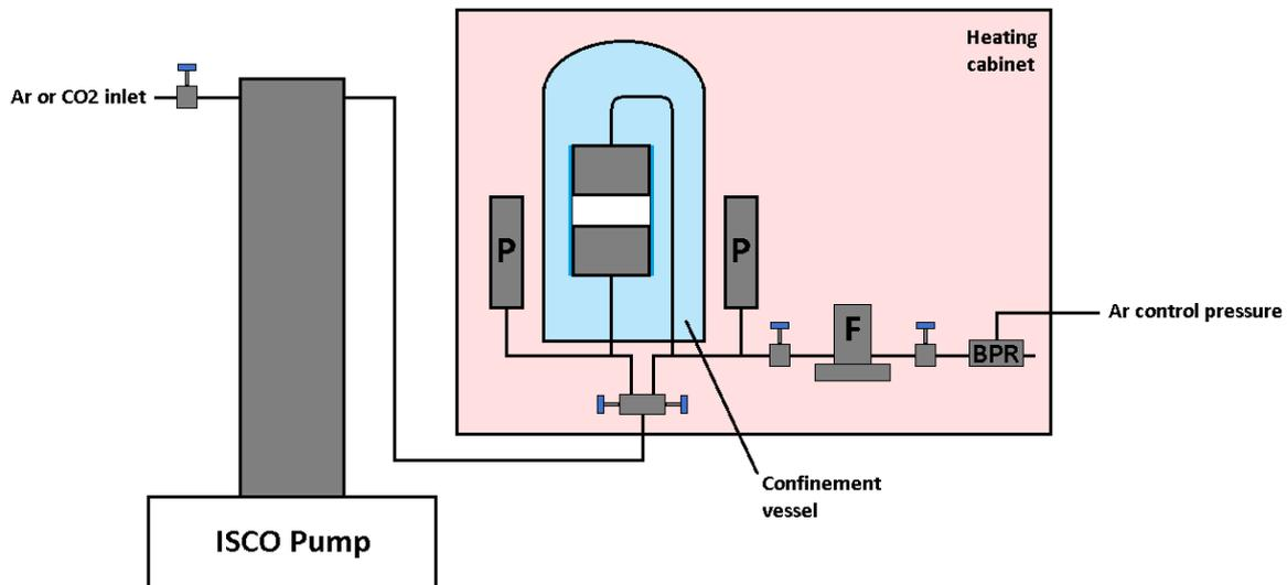
**Figure 1** Schematic drawing of the permeability apparatus used in the reported measurements. The Pump used is an ISCO 100DX.
