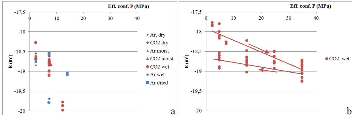
**Figure 2** Transient pulse permeabilities ( $m^2$ ) plotted versus effective confining pressure (MPa), measured on: a) Sample 2; a pure smectite tablet, subsequently tested dry, moist, wet, and dried. b) Sample 4; a quartz-smectite tablet measured wet (as the dry permeability was too high to measure). The trend lines show the change in permeability with increasing and decreasing confinement, as indicated by the arrows.
