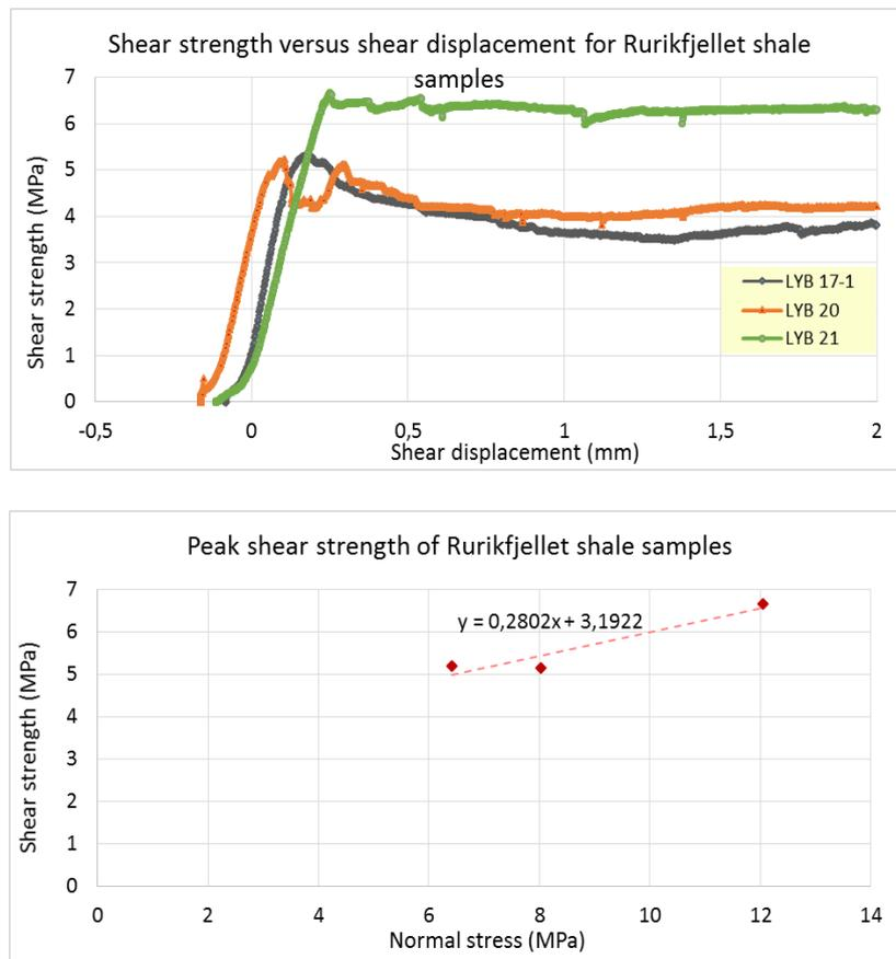
**Figure 4** Results of direct shear tests on three shale samples from Rurikfjellet Formation, Svalbard. (a) Shear strength versus displacement and (b) shear strength versus normal strength with an interpreted failure line.
