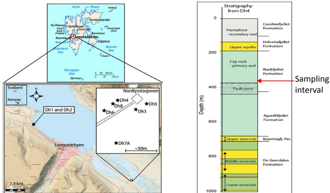
**Figure 1** Location of boreholes drilled at the Longyearbyen CO<sub>2</sub> storage site, Svalbard, northern Norway (left) and stratigraphy column in borehole Dh4 along with the sampling interval for this study.
