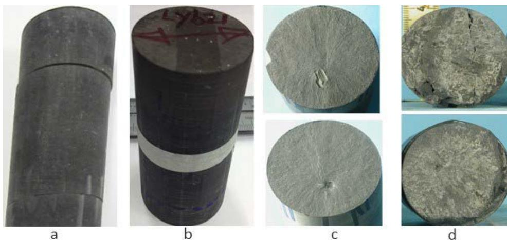
**Figure 3** Shale cores from Svalbard used in this study. (a) discing of shale core along the bedding plane, (b) a test specimen separated along bedding plane and attached and taped together, (c) surface of the fracture before shearing and (d) after shearing in the direct shear box.
