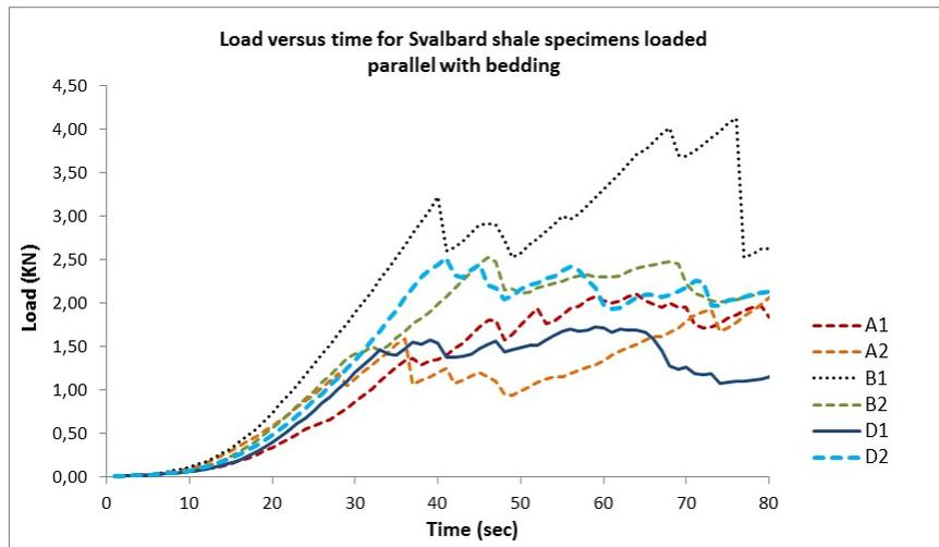
**Figure 3** Load versus time for shale samples loaded parallel with bedding plane. Sample B1 (black-dashed line) reaches the first peak load and fails at around 40 seconds. Further failure development results in peak loads that are higher than the failure peak. A similar trend is also observed for other samples where post-failure peaks are almost as big as the failure peak.
