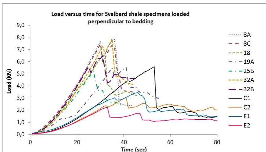
**Figure 4** Load versus time for shale samples loaded perpendicular to bedding plane. Failure of samples is indicated by the first peak load followed by a sudden drop. After the drop, sample bear some loads but never reaches the same level as the failure peak.
